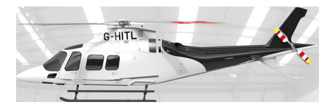
Note: Leonardo list the specification in both VFR and IFR configurations, this aircraft is confirmed as Single Pilot IFR with 4 axis auto pilot
